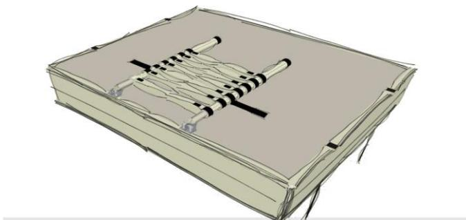
7. Choose a proper direction according to the roof bar of your car to install the tent on your car. Tighten all bolts and nuts carefully when correct positioned.
