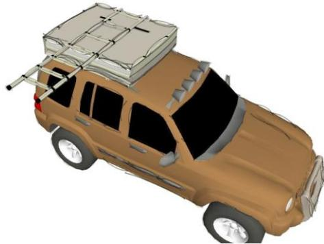
3. Set up the tent by dragging the ladder, adjust the position of the ladder.
